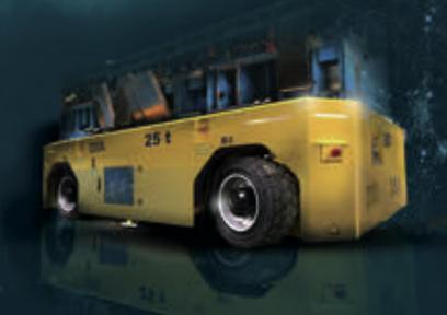
Rhino movers for handling loads with remote control from 1 ton up to 70 tons.
